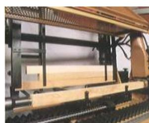
Loader and clamping device
